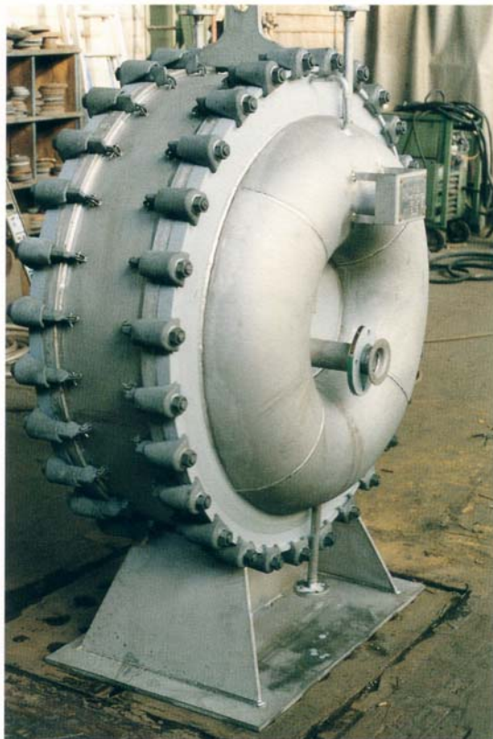
Spiral heat exchanger for disinfection with heated cover
