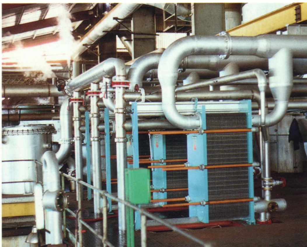
Three Wide-gap plate heat exchangers with automatic backflushing heat mixed juice with boiler vapour at the Industrielle Sucrière de Bourbon on La Réunion.
