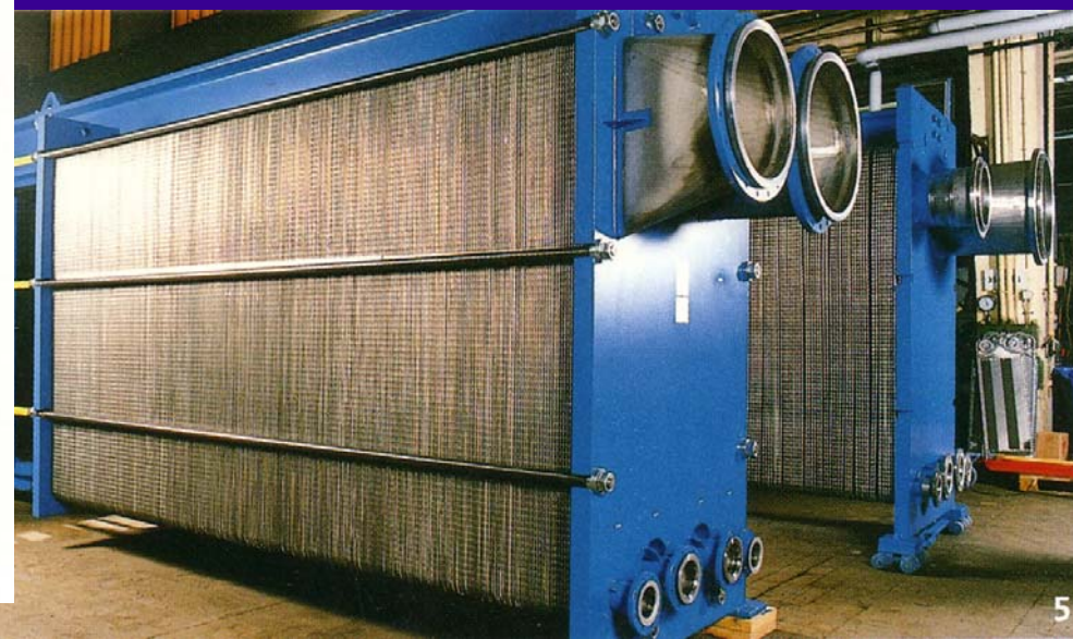
Three Wide-gap plate heat exchangers with automatic backflushing heat mixed juice with boiler vapour at the Industrielle Sucrière de Bourbon on La Réunion.
