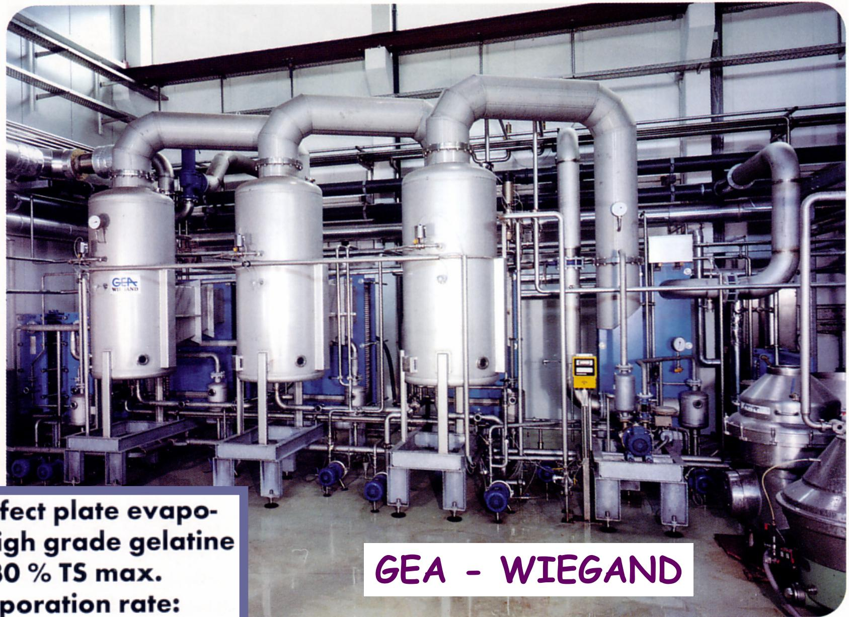
**Multiple effect plate evaporator for high grade gelatine from 4 to 30 % TS max.
