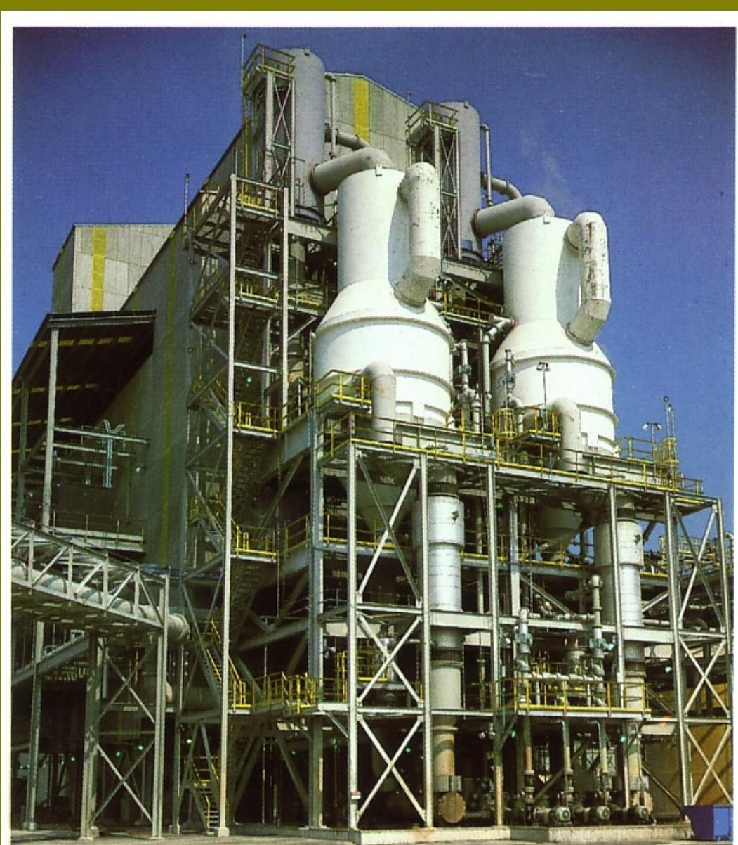
Two-stage, forced-circulation evaporator used to concentrate wet process phosphoric acid
